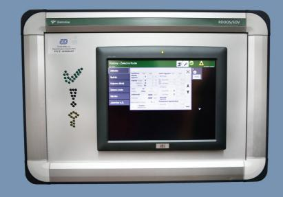
Control board RD00S/EOV is a main unit of DOOS system. Allows connection to control devices such as lighting control units, programmable controllers (PLC) of rail switch heating cabinets, CCTV systems, object serucity equipments and others control units. Communication to dispatch centers and local administrators complies to TS2/2008 regulation (Remote diagnostics of technological systems of Railway infrastructure).
