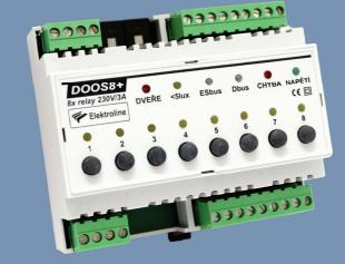
D00S8+ is illumination control unit with 8 separately controlled relay outgoings. Unit is designed for switching the lighting circuits or any power circuits which may be controlled and their status could be monitored.
