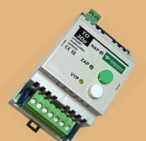
T05Dp (T03Dp) is main unit of remote control system. Is controlled by a processor and allows control of motor drive by local buttons, or by two types of remote control – by binary inputs or by RS485 data bus and is addressable. A block of local control ensures a central switch located on the T0ZD source front panel installed in all control boards.
