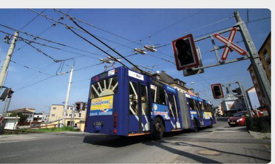
New type of TBUSxTRAM (15°-65°) crossings without interruption of electrical supply is perfectly silent and ensure vehicle's sustained passage with current.
