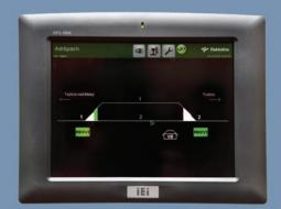
Parameters of control boards equipped with 8" or 19" touchscreen are identical. Difference is only on board design and dimensions. Type of control board may be selected with regard to quantity of operated devices for their comfortable viewing.
