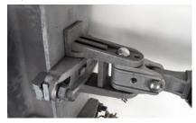
Together with positive-locking connections of pole cross-arms and diverse connection parts, with no fastenings, the range of mounting variants is extended with the least variety of parts.
