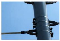
Reusable swivel joint mountings with steel bands on circular or profile section poles, using Lindapters or U-bolts, meet individual customer requirements.
