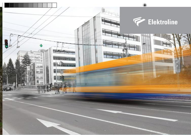
AN INCREASE IN ENERGY DEMAND IS EXPECTED WHILE USING HYBRID BATTERY TROLLEYBUSES. WHEN THESE BUSES RETURN TO THE CATENARY THEY CONSUME ENERGY NOT ONLY FOR NORMAL OPERATIONS, BUT ADDITIONALLY FOR ON-BOARD BATTERY CHARGING. THE TOTAL CONSUMPTION OF TROLLEYBUSES IS THE SUM OF THE BATTERY CURRENT AND TRACTION CURRENTS.
