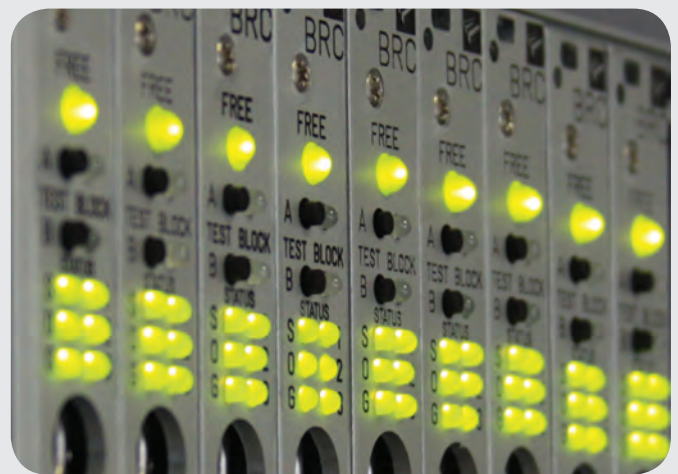
Track circuit electronic units BRC
