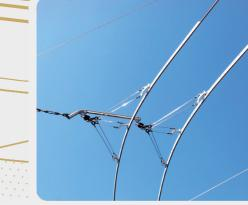
The curve clamps are designed for high-speed vehicles.
